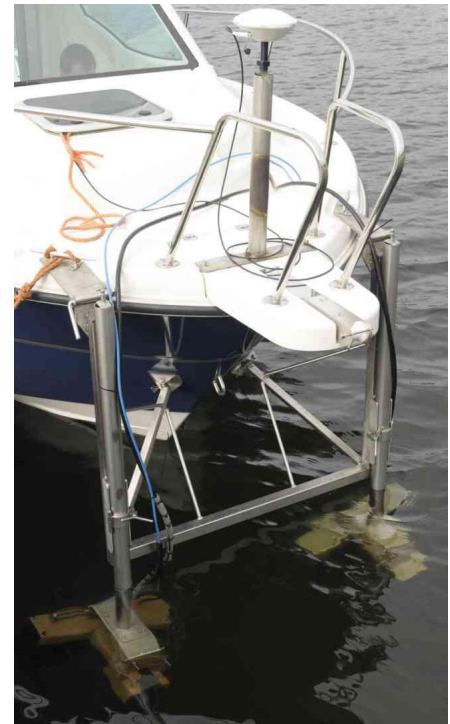
Fig 1: 7 m long survey vessel "Karnic" equipped with 2 R2Sonic Sonic 2024, Ixsea Octans G4, Stema Systems GNSS960, Qinsy8.0
